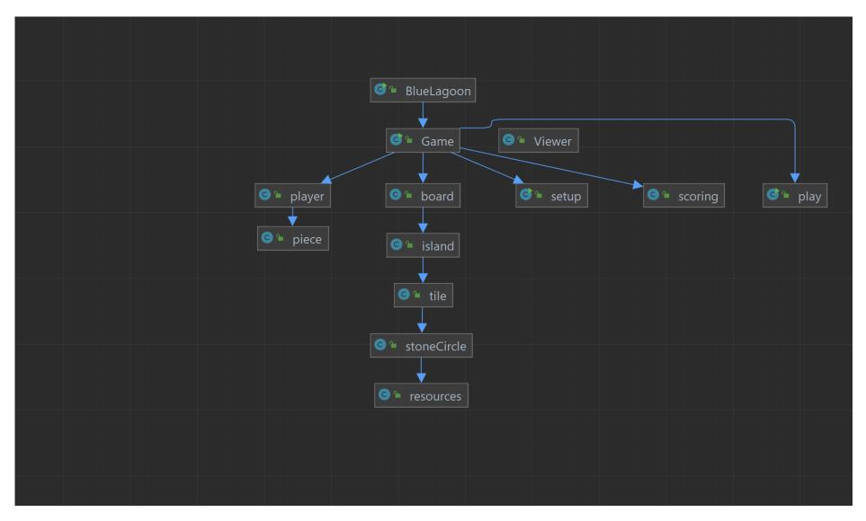
This class diagram (made in IntelliJ) is a visual representation of the new classes in our design skeleton and their relationship to the other project classes at this point in time. Arrows have been added to aid in illustration.
